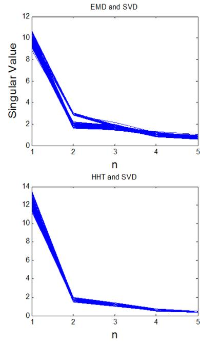
**Figure 6.** The singular value clusters of rolling element fault signal.
