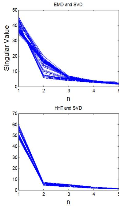
**Figure 5.** The singular value clusters of outer-race fault signal.
