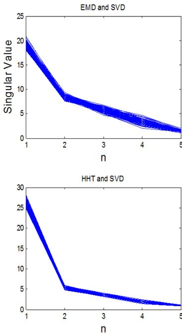
**Figure 4.** The singular value clusters of inner-race fault signal.
