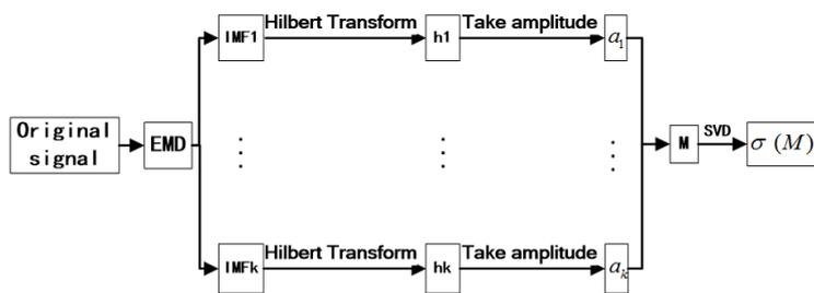
Figure 1. Flowchart of obtaining the feature vector.
