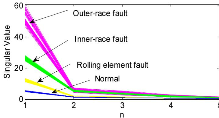
**Figure 7.** The singular value clusters of different fault model.
