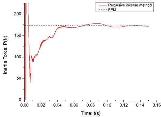
**Figure 2.** The experiment identification result ( $c=10\text{m/s}$ ).
