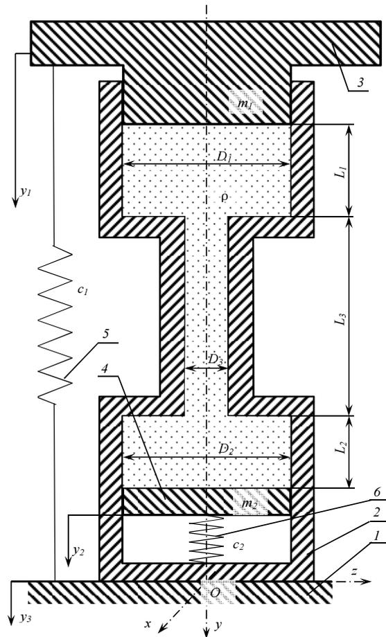
**Figure 1.** Design scheme of hydraulic mount.
