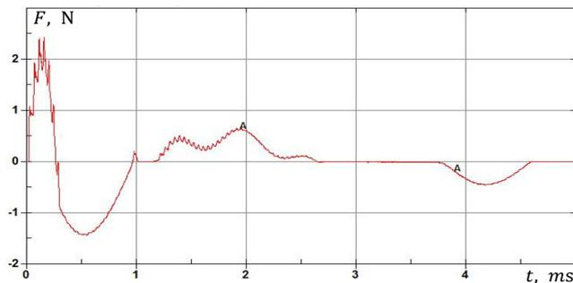
**Figure 2.** Resultant force acting on the base.
