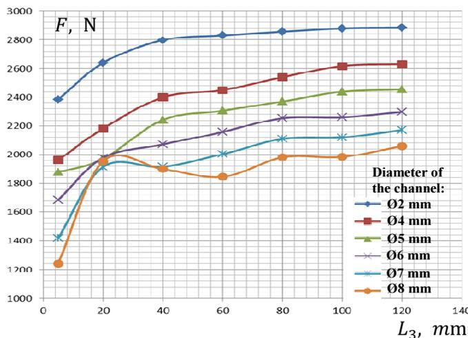
**Figure 3.** Peak values of dynamic force  $F$  acting on the base depending on the channel length  $L_3$  and diameter.
