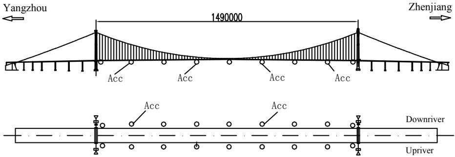
Fig. 3. Vibration monitoring sections in the main girder
