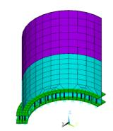
Fig. 4. Detail of mesh – bottom rims
