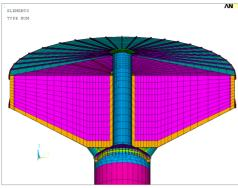
Fig. 3. Detail of mesh - tank bottom
