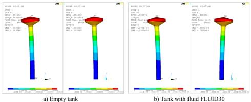
Fig. 5. First bending mode
