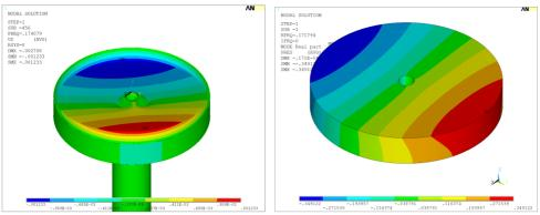
a) Fluid - FLUID80 – displacement field b) Fluid - FLUID30FREE – pres. field **Fig. 8.** Eigen mode corresponding to 1<sup>st</sup> eigen mode of fluid movement
