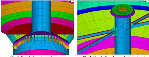
Fig. 1. Detail of mesh - tank bottom
