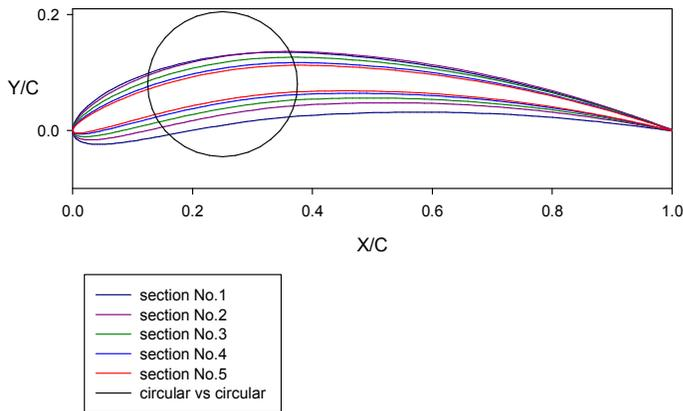
Fig. 3. Stack-up of the five optimum airfoils
