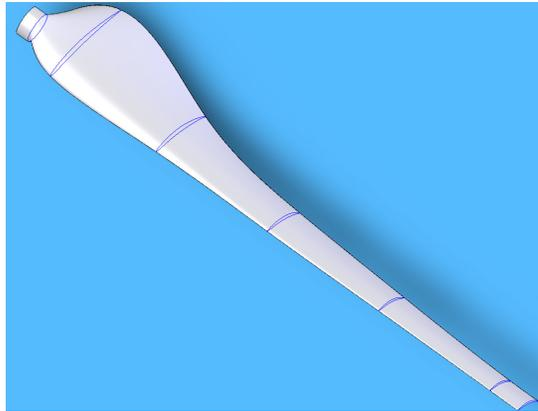
**Fig. 5.** 3-D model of the optimized blade
