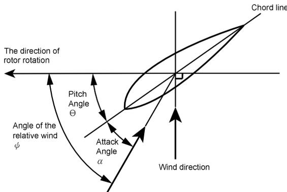
**Fig. 1.** Orientation of an airfoil
