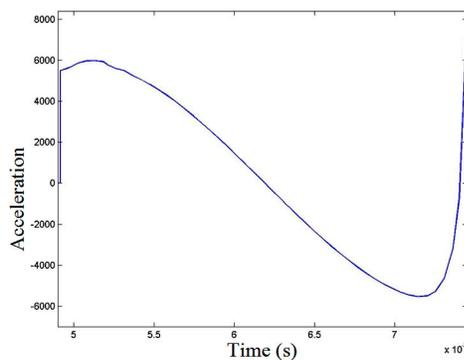
Fig. 9. The valve acceleration profile in proposed EMV
