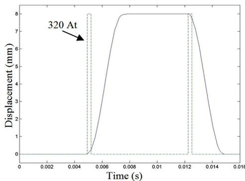
Fig. 7. Displacement and current profiles for EMV
