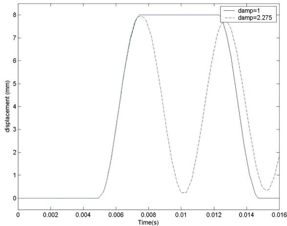
Fig. 14. The effects of damping coefficient on EMV
