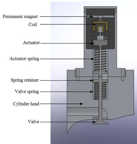
**Fig. 1.** Structure of hybrid PM/EM EMV
