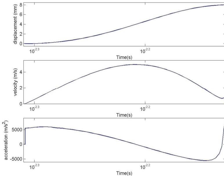
**Fig. 11.** The valve acceleration profile in proposed EMV
