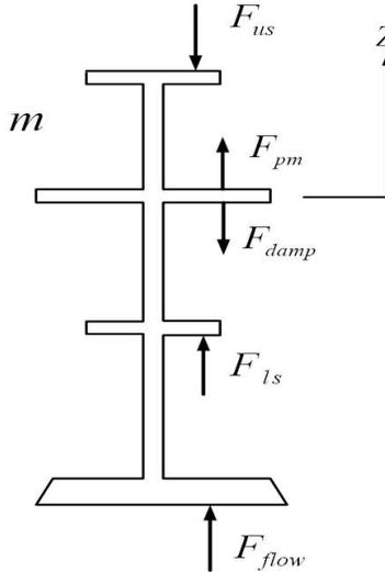
Fig. 4. The free body diagram of armature and valve in EMV
