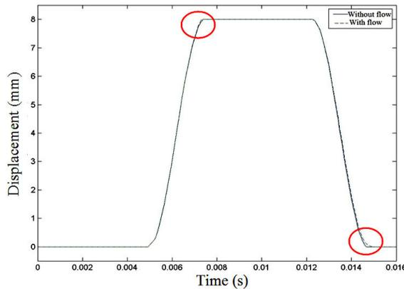
Fig. 13. The effects of gas flow force on valve displacement
