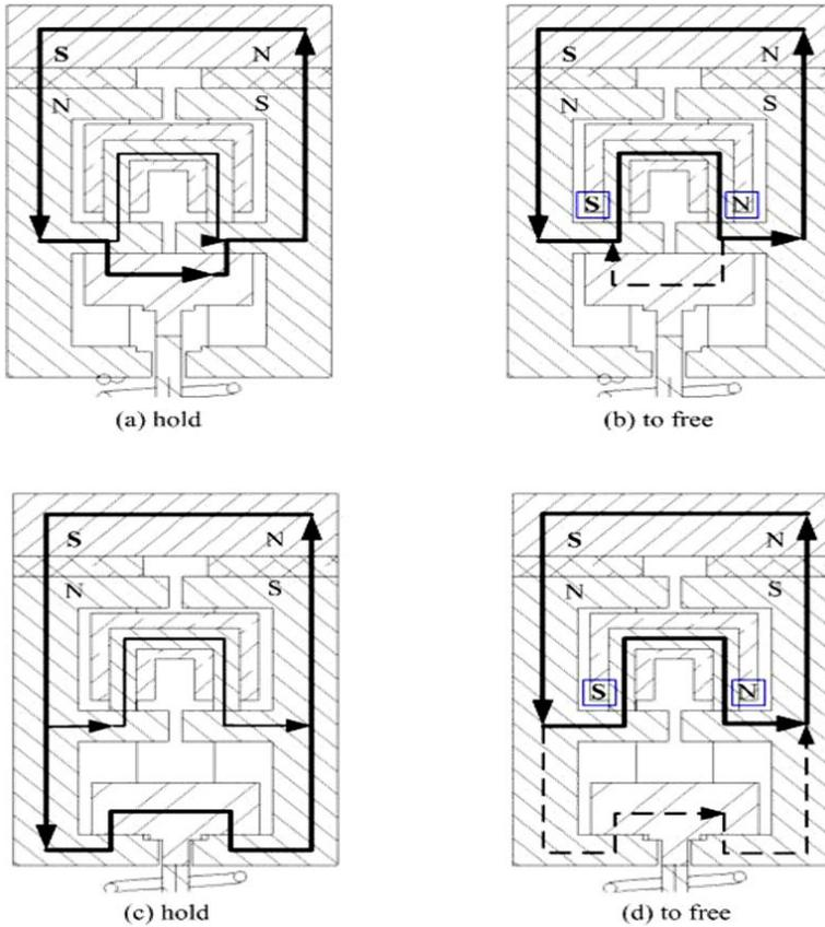
Fig. 2. The proposed EMV operation principle
