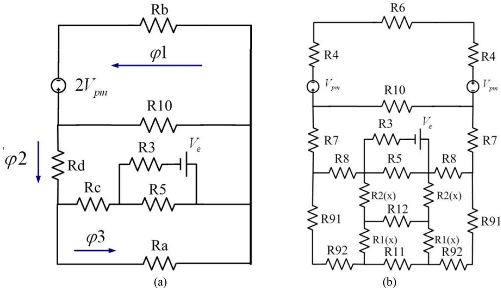
Fig. 5. (a) The electromechanical subsystem in EMV system, (b) the simplified magnetic circuit
