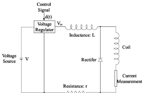
Fig. 3. The electrical subsystem of EMV
