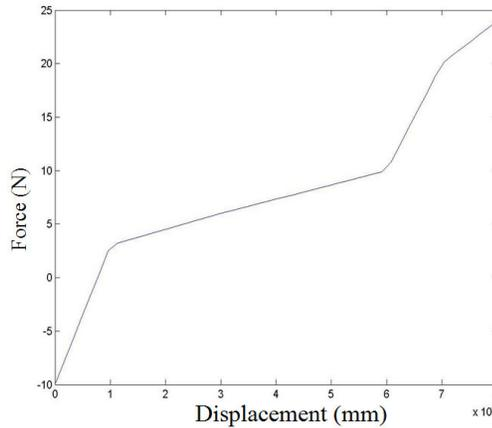
Fig. 12. The gas flow force from closed to open positions
