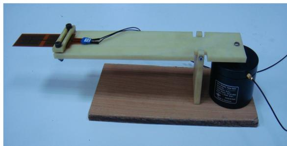
**Fig. 2.** Experimental platform of vehicle-vibration harvesting output power for the NQ45N smart material
