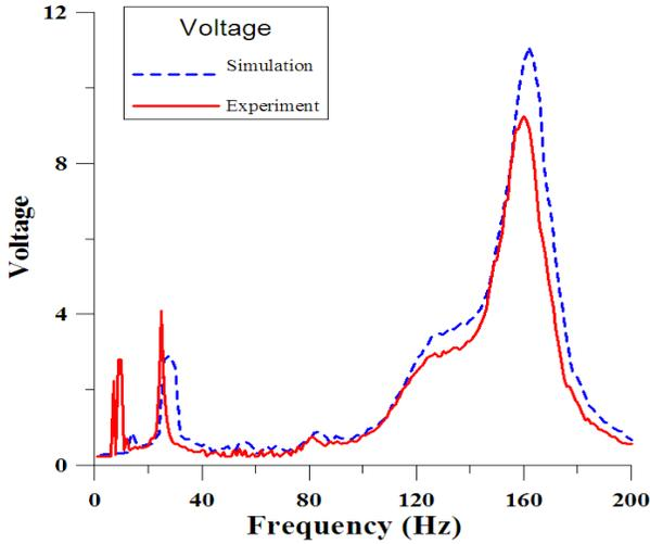
**Fig. 7.** Characteristic comparison of output voltage versus vibrating frequencies for the NQ45N smart material through the ANSYS harmonic simulation and experiment
