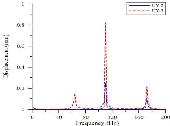
Fig. 4. Optimum analysis of bending displacement in relation to vibrating frequencies for the QuickPack NQ45N smart material through ANSYS simulation (Harmonic analysis)
