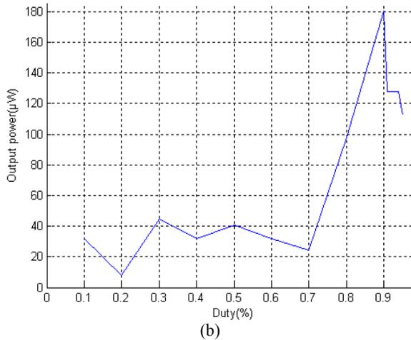
**Fig. 8.** (a) Testing circuit of harvesting output power based on a buck converter for the QuickPack NQ45N material, and (b) characteristic of harvesting output power
