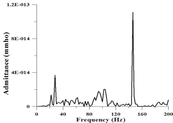
Fig. 5. Characteristic analysis of admittance versus vibrating frequencies for the QuickPack NQ45N smart material through ANSYS software
