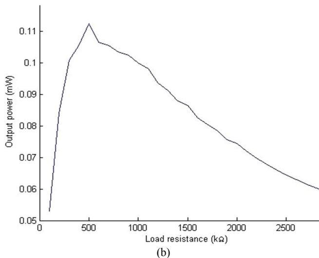
**Fig. 6.** (a) Testing circuit for loading output, and (b) output power characteristic with various loading resistance
