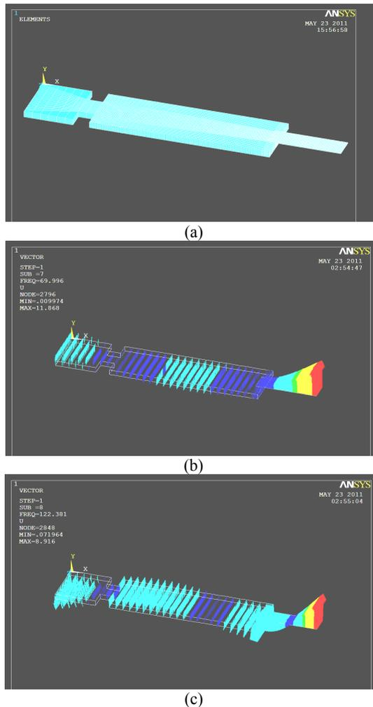
**Fig. 3.** (a) Modeling smart materials by ANSYS software, (b) seventh natural mode (at 70 Hz), and (c) eighth mode (at 122 Hz) by ANSYS modal analysis
