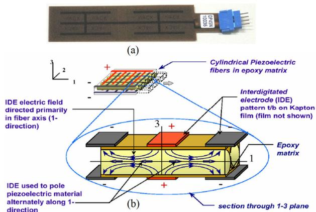
**Fig. 1.** (a) Appearance of QuickPack smart material (Model-NQ45N), (b) Apparatus of electrodes and electrical field applied on electromechanical coupling effects (adopted from Mide Technology Corporation)
