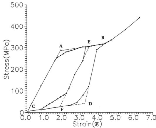
Fig. 1. The strain-stress curve of SMA
