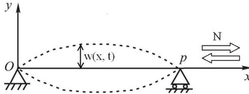
Fig. 2. The model of SMA simply supported beam in axial stochastic excitation
