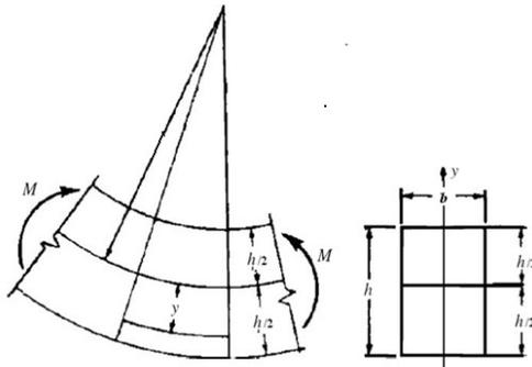
Fig. 3. The cross-section and curvature of the assumed beam
