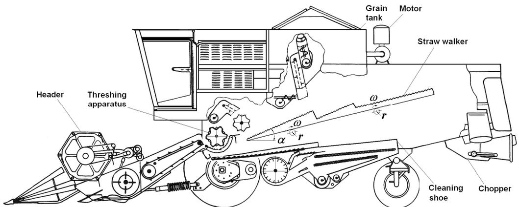
**Fig. 1.** Combine harvester with tangential threshing apparatus and straw walker:  $\alpha$  – the inclination angle of walker surface;  $r$  – crankshaft radius;  $\omega$  – angular velocity
