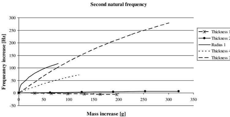
**Fig. 9.** Second eigenfrequency dependency on mass increase
