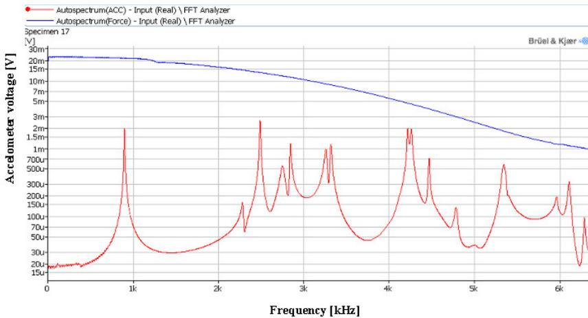
Fig. 4. Typical graph of brake drum frequency response
