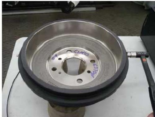
**Fig. 3.** Impact hammer test measurement setup
