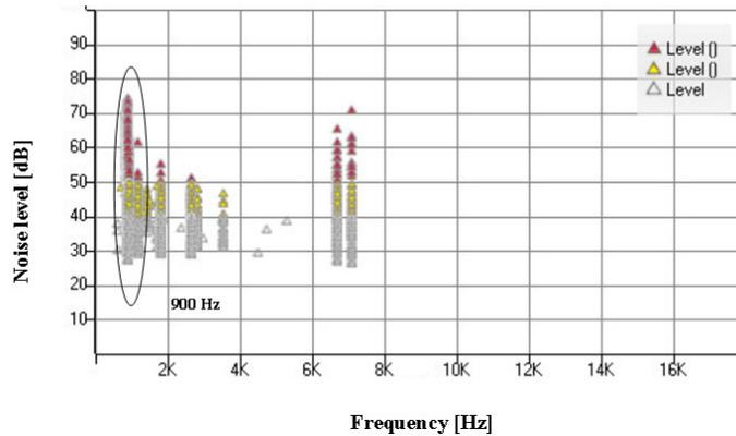
**Fig. 2.** Noise results of the considered rear brake drum
