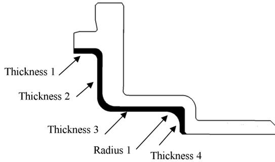
**Fig. 7.** Possible brake drum modifications
