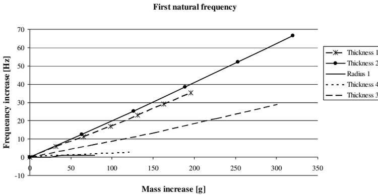
**Fig. 8.** First eigenfrequency dependency on mass increase
