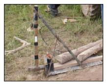
Fig. 3. Plate used for excitation of shear waves
