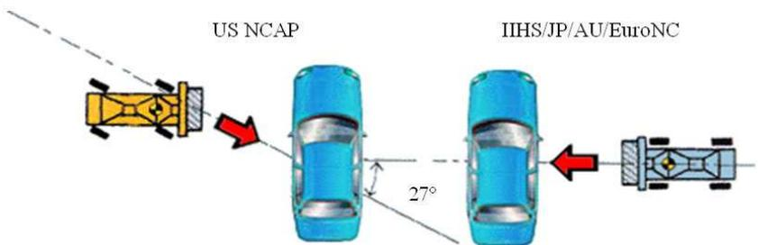
Fig. 2. Side impact test according to different safety requirements. R-point equal for hit point for 95<sup>th</sup> percentile male
