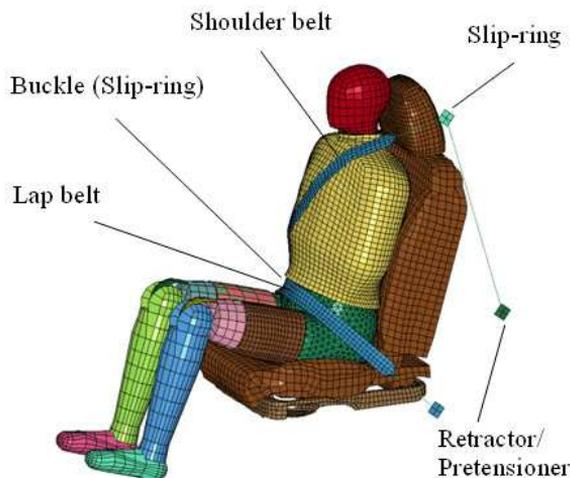
**Fig. 4.** Belted USSID model
