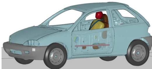
Fig. 3. General Motors GeoMetro FEM
