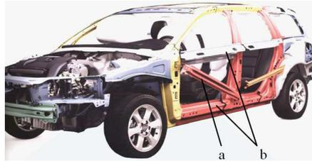
Fig. 1. Car side door design: a - anti-intrusion beam, b - upper and lower crossbars
