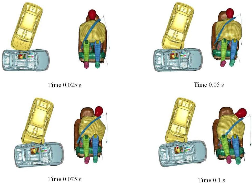
**Fig. 5.** Vehicles and dummy kinematics during side impact
