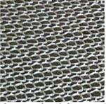
Fig. 4. Custom made glass fiber knitted fabric sample is ready for composite reinforcement (left picture); fabric's structure (right picture)
