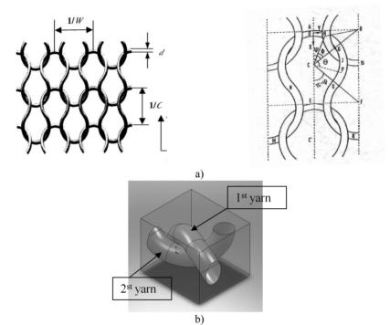
Fig. 7. a) Schematic diagrams of knitted fabric structure [10]; b) fabric's unit cell
