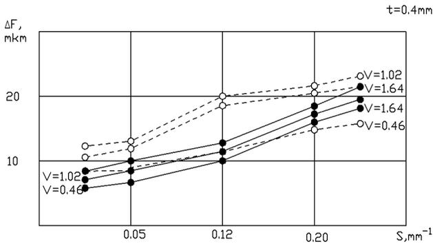
**Fig. 11.** Dependence of deviations of the cross-section roundness  $\Delta F$  on the feed rate ( $t = 0.4$  mm):
