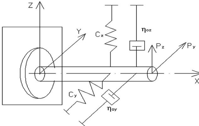
**Fig. 1.** Principal diagram of the dominating oscillating system in the process of boring:  $C_y$ ,  $C_z$  are coefficients of rigidity of the generalized shaft along axis  $Y$  and  $Z$ , respectively;  $\eta_{oy}$ ,  $\eta_{oz}$  are generalized resistance (damping) coefficients along the corresponding axis
