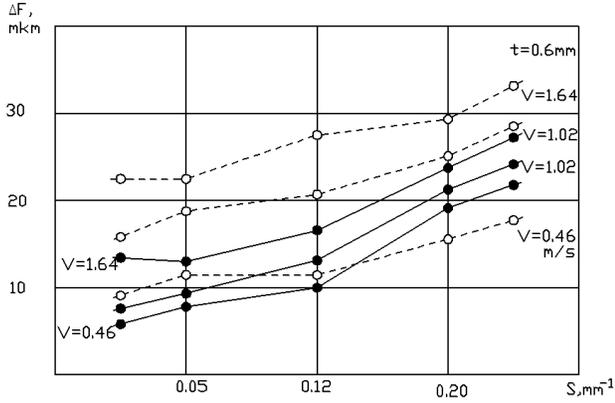
**Fig. 10.** Dependence of deviations of the cross-section roundness  $\Delta F$  on the feed rate ( $t = 0.6$  mm):
