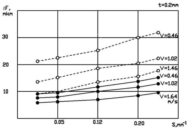
**Fig. 12.** Dependence of deviations of the cross-section roundness  $\Delta F$  on the feed rate ( $t = 0.2$  mm):
