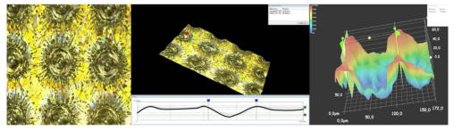
Fig. 7. The topography of nanocrystalline surface of the padding weld after laser texturing in order to form oil microcontainers essential in tribological processes
