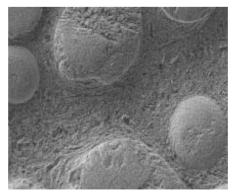
Fig. 3. Spheroidal carbides as components of standard padding materials [6]
