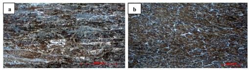
Fig. 1. The structure of the joint: a) after laser welding; b) after laser welding with the use of TiCN + Cu nanopowder [5]
