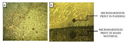
**Fig. 5.** Microstructure of the padding weld performed with the laser technique: a) zone of the padding weld material, b) penetration zone with the visible imprints of the microhardness tester at a load of 100G
