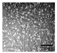
Fig. 2. Microstructure of EnDOtec TO \* 390 padding wire [6]
