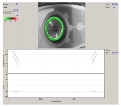
Fig. 11. Displacement distribution on the actuators top surface
