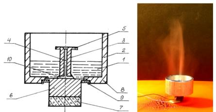
**Fig. 6.** Half size view schematics and a picture of real working device: 1 - liquid, 2 - vessel, 4, 10 - capillary, 5 - spraying surface, 6 - actuator, 7 - piezoelement, 8 - vessel with liquid, 9 - fastening
