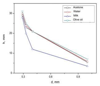
Fig. 5. Liquid rise, level dependence on capillary diameter
