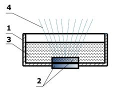
Fig. 2. High-frequency ultrasonic dispersion: 1 - tank, 2 - piezoelements, 3 - liquid, 4 - sprayed liquid
