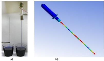
**Fig. 4.** Colored water raises up in a capillary tube under longitudinal vibrations (a) and a model of the same system made using FEM method (b)
