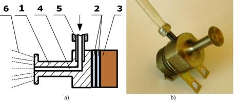
**Fig. 3.** Schematics (a) and real view (b) of sprayer: 1 - transducer, 2 - piezoelement, 3 - counterweight, 4 -flow channel, 5 - inlet port, 6 - sprayed liquid
