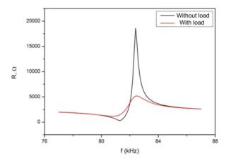
Fig. 7. Impedance-frequency characteristics of piezoelectric actuator
