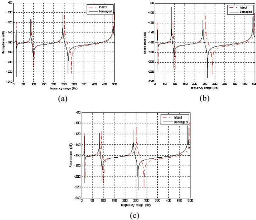
**Fig. 2.** FRF of intact and damaged beam at a typical measurement point:
