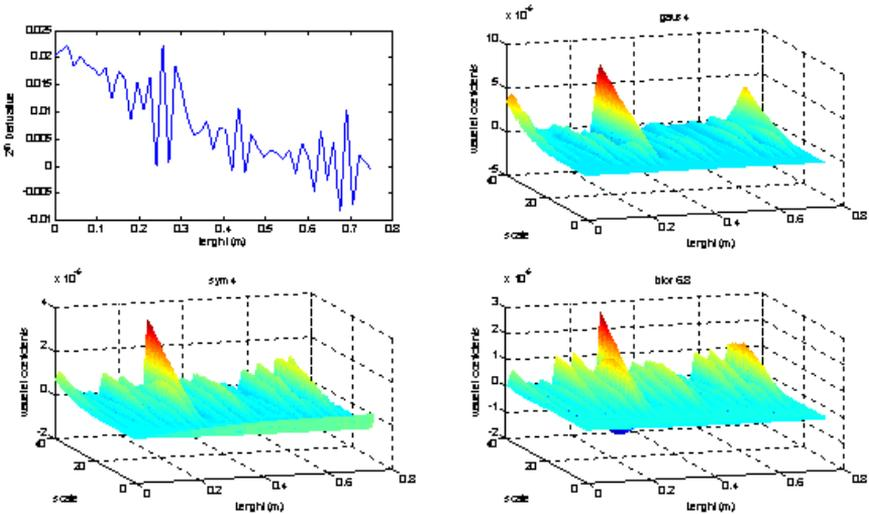
Fig. 8. Wavelet coefficients for 40% damage with  $\rho = 0.0001$  (Contaminated mode shapes)
