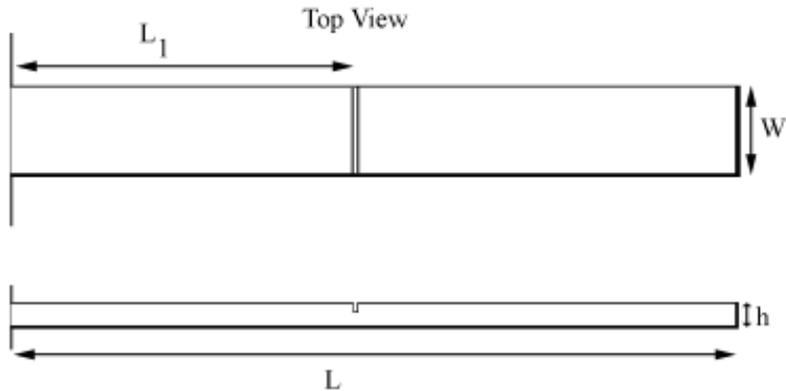
Fig. 1. Layout of cantilever beam with a crack
