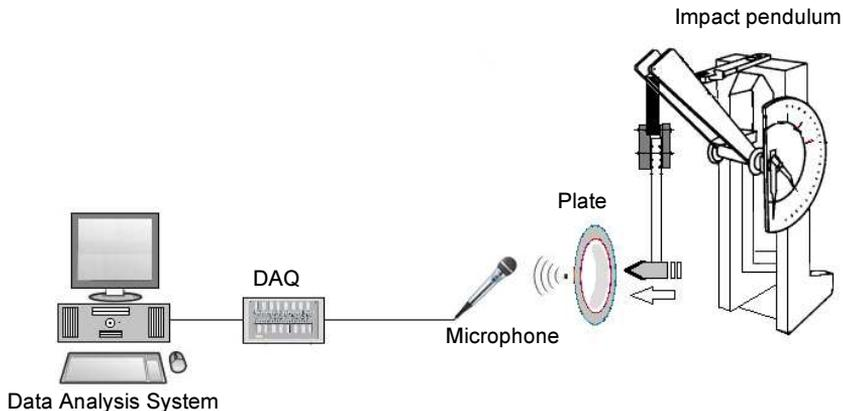
Fig. 1. Data acquisition and measurement system [1]
