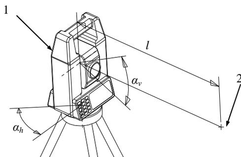
**Fig. 1.** Point position (coordinates) determination principle by measuring geodetic instrument:
