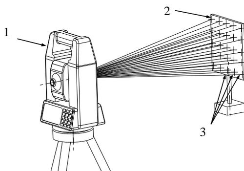
**Fig. 2.** Measuring of point cloud of plate surface: 1 – geodetic angle instrument (tachometer),
