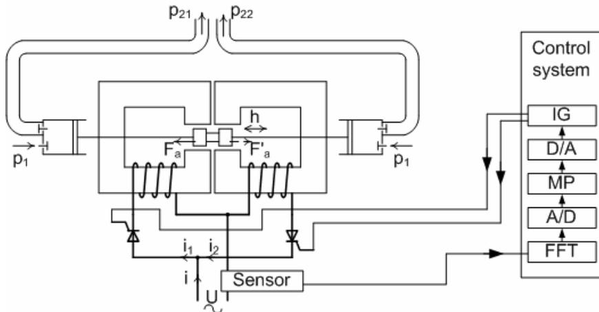
**Fig. 1.** Double-sided springless LOEM with pulsating current source with the piston compressor load. Where FFT is Fast Fourier Transform block, A/D – analog/digital converter, MP – microprocessor or microcontroller, D/A – digital/analog converter, IG – control impulse generator
