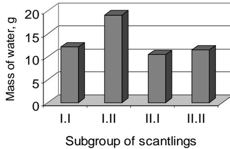
**Fig. 8.** The average water quantity in scantlings: I.I – across and along the fiber, without vibration application, I.II – with vibration application, II.I – across the fiber, without vibration application, II.II – with vibration application
