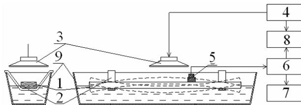
**Fig. 1.** The scheme of measuring setup: 1 – wood assortment and its bending; 2 – elastic elements; 3 – acoustic vibrator; 4 – vibration generator; 5 – vibration detector; 6 – measuring instrument; 7 – oscilloscope; 8 – phase meter; 9 – water container
