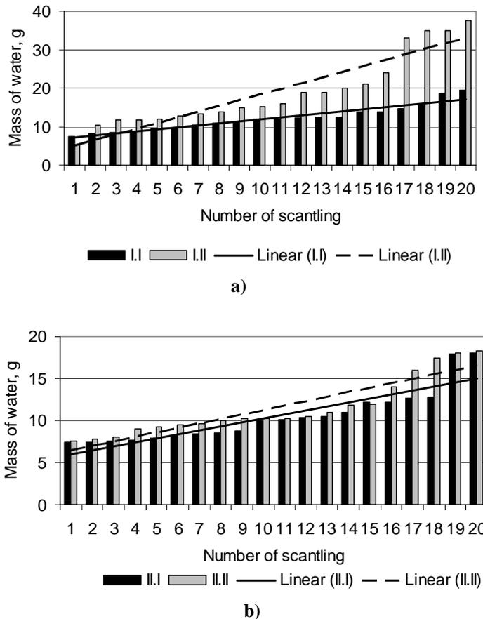
**Fig. 7.** The comparison of water quantities contained in scantlings: (a) – along and across the fiber; (b) – across the fiber; I.I and II.I – scantlings without vibration application, I.II and II.II – scantlings with vibration application
