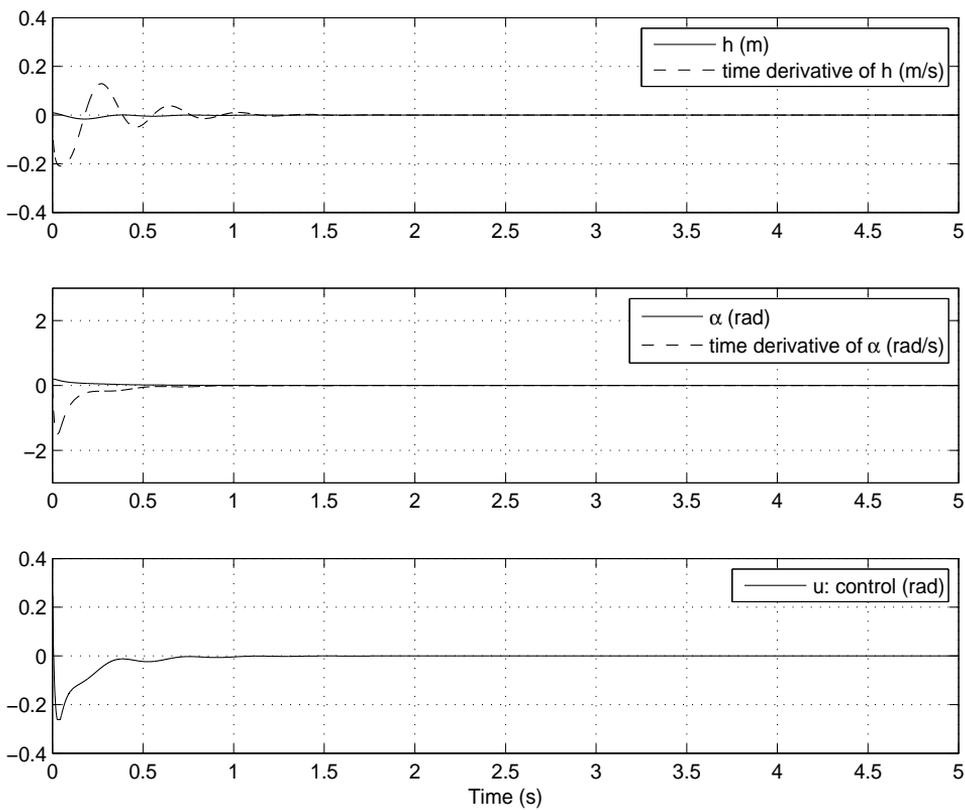
**Fig. 3.** Wing vibration stabilization for freestream velocity  $V = 30 \text{ m/s}$ , and initial conditions:
