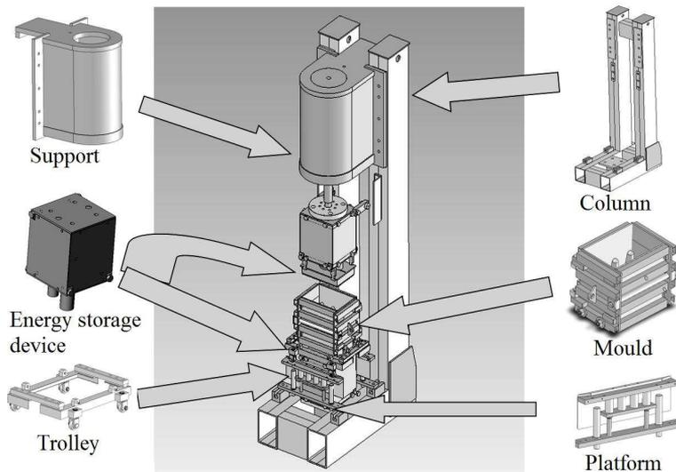
**Fig. 1.** Two-sided vibro-impact press
