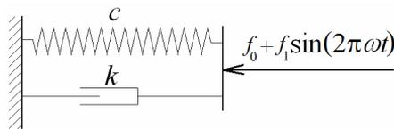
**Fig. 11.** The simplest Kelvin-Voigt dynamic model of vibropressing
