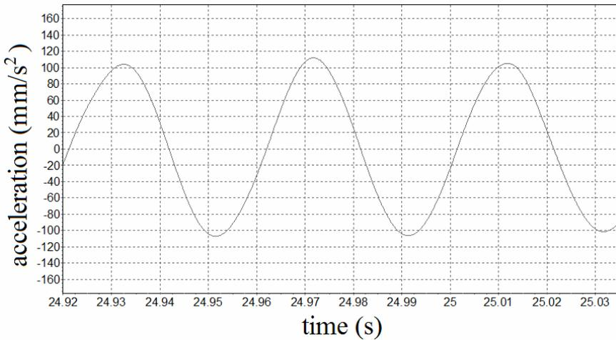
**Fig. 9.** Numerically calculated plunger acceleration
