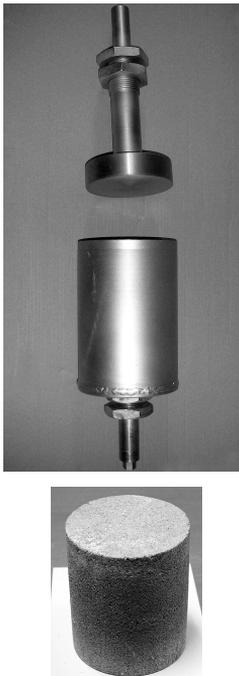
**Fig. 2.** Pressing plunger, mold and compacted concrete block specimen
