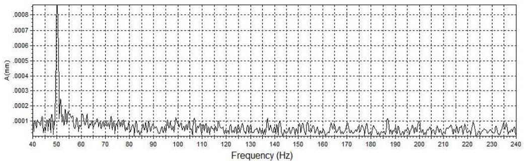
**Fig. 6.** Fourier spectrum of displacement oscillations with 50 Hz pressing force
