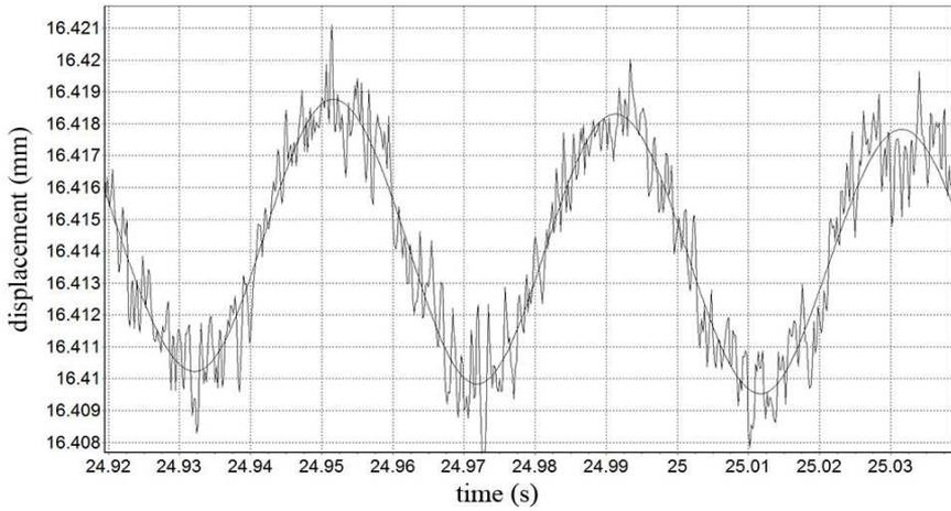
**Fig. 8.** Registered and smoothed plunger displacement graphs
