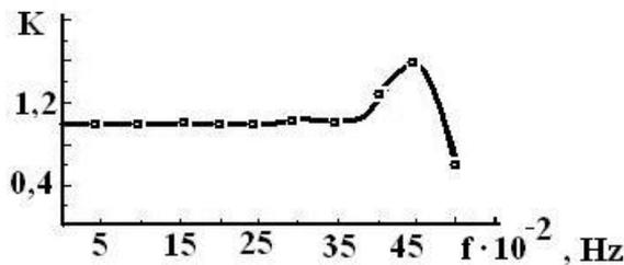
**Fig. 6.** Transfer characteristic of the resonance table disk
