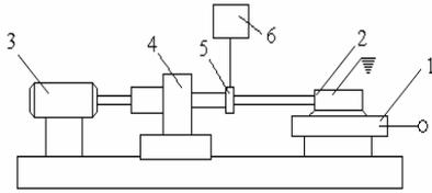
**Fig. 2.** Scheme of the appliance for measurement the fixing loading of fixing an item to the working table
