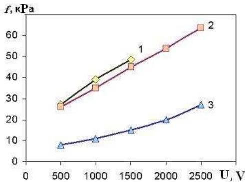
**Fig. 3.** Dependence of the specific fixing force in fixing an aluminium item on the voltage of the electric field: 1 – the thickness of dielectric coating of the electrode 35, 2 – 50, 3 – 75  $\mu\text{m}$
