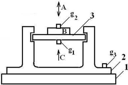
**Fig. 5.** A sketch of the resonance table for the investigation of the coefficient of transmitting mechanical loadings by the ER method of fixing items: 1 – vibrostand platform; 2 – frame; 3 – resonance disk; A – the direction of vibrations; B – fixing table with a sample, C – the direction of tightening of the resonance disk.;  $g_1$ ,  $g_2$ ,  $g_3$  – sensors to measure acceleration.
