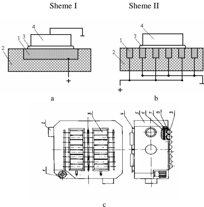
**Fig. 1.** Schemes of fixing items to electrodes through a layer of ER glue: a – plane item with a conductive surface, b – item with a dielectric plane surface, c – cylindrical items with conductive surfaces - 1, terminal block; 2, current protection unit; 3, capacitors; 4, plate for making soldered terminals of capacitors; 5, body; 6, insulator; 7, insert; 8, ER glue
