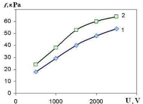
**Fig. 4.** Dependence of the fixing force in fixing an asbestos cement item on the voltage of the electric field: 1 – without a coating, 2 – with a lacquer coating
