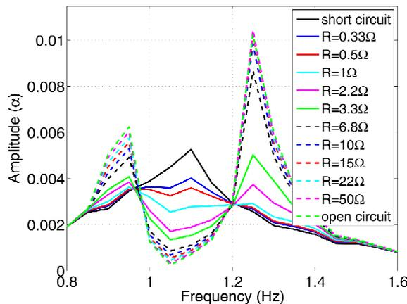
**Fig. 3.** Numerical simulations: normalized amplitude of the modal coordinate  $\alpha$  versus excitation frequency. Several values of resistance  $R$  are tested
