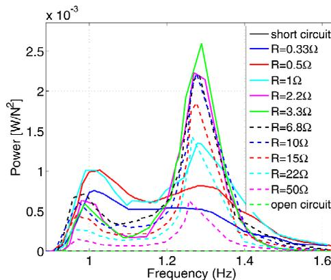
**Fig. 7.** Experimental results: normalized power harvested versus excitation frequency. Several values of resistance  $R$  are investigated
