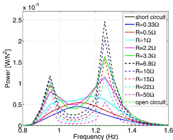
**Fig. 4.** Numerical simulations: normalized power harvested versus excitation frequency. Several values of resistance  $R$  are tested
