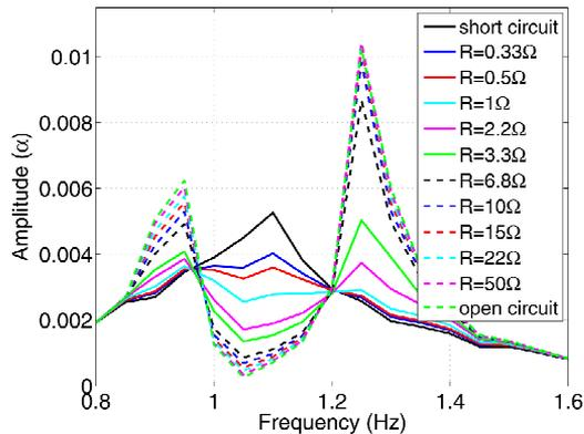
**Fig. 6.** Experimental results: normalized amplitude of the modal coordinate  $\alpha$  versus excitation frequency. Several values of resistance  $R$  are tested
