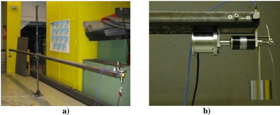
**Fig. 5.** Experimental setup: a) bridge mock-up equipped with pendulum-alternator actuator and eccentric mass shaker, b) detailed view of the pendulum-alternator actuator
