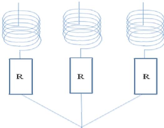
**Fig. 2.** Electrical scheme of the alternator connected to a resistive load
