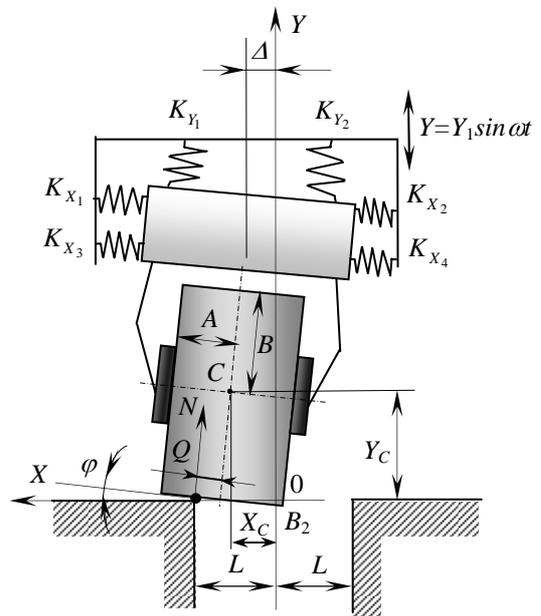
**Fig. 2.** Dynamic model of vibratory alignment
