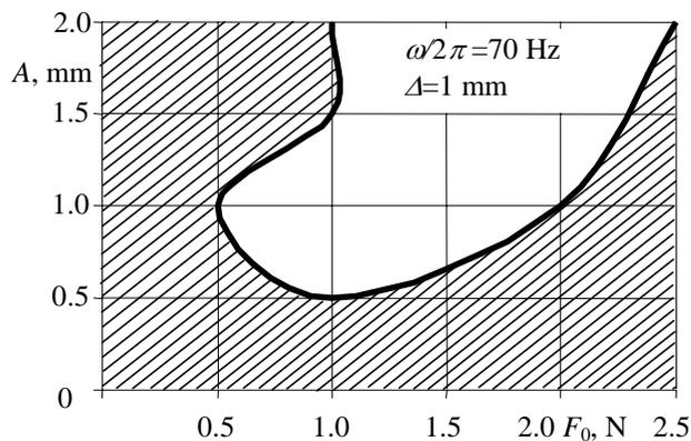
Fig. 7. Area of stable alignment of rectangular cross-section parts (unhatched) depending on excitation amplitude and initial pressing force
