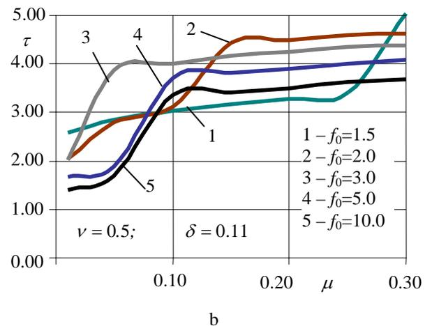
**Fig. 3.** Dependencies of parts alignment duration on: a – initial pressing force  $f_0$ ; b – friction coefficient  $\mu$
