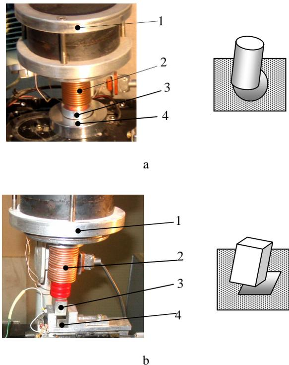
**Fig. 5.** Experimental setup for cylindrical (a) and rectangular cross-section (b) parts alignment
