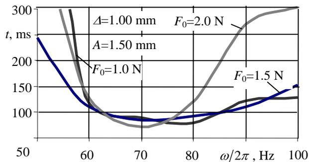
Fig. 6. Dependence of rectangular parts alignment duration  $t$  versus excitation frequency
