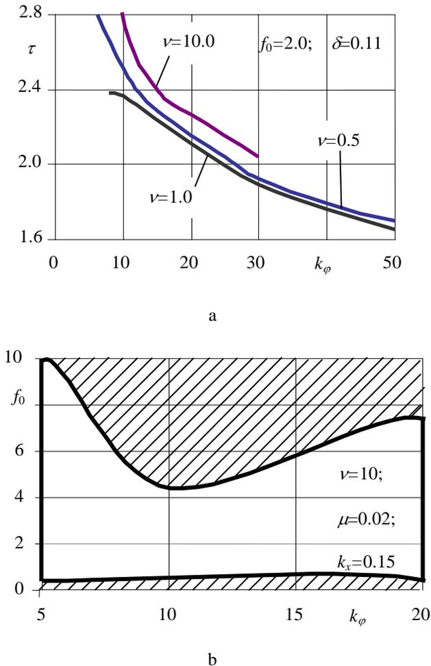
**Fig. 4.** Dependencies of parts alignment duration  $\tau$  on parameter  $k_\varphi$  (a); defined area of stable alignment of the parts (unhatched) depending on parameters  $k_\varphi$  and  $f_0$  (b)
