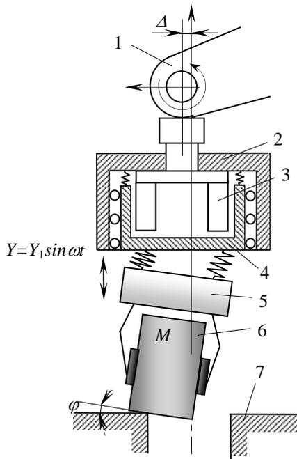
**Fig. 1.** Scheme of robotized assembly: 1 – robot arm; 2 – platform of electromagnetic vibrator; 3 – electromagnet; 4 – gripper holder; 5 – gripper; 6 – shaft; 7 – bushing
