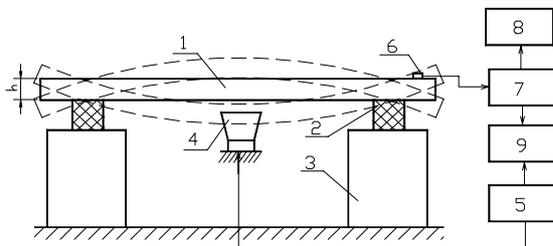
**Fig. 1.** Set-up for testing wood articles: 1 – wood assortment and its mode; 2 – elastic elements; 3 – massive supports; 4 – acoustic vibrator; 5 – generator of electric oscillations; 6 – sensor; 7 – measuring device; 8 – oscillograph; 9 – phasometer
