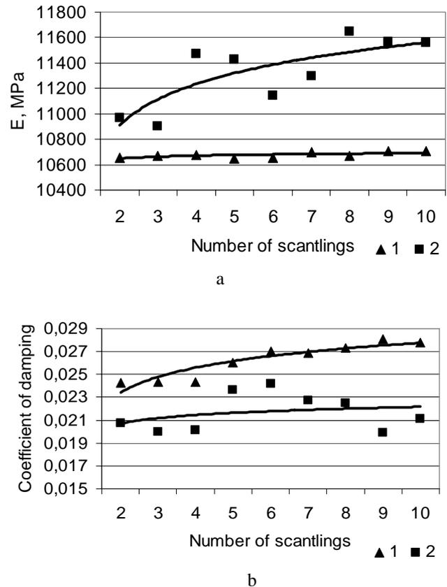
Fig. 3. Consistent patterns of varying average modulus of elasticity (a) and damping coefficient (b) of oak wood scantlings, and of first-type panels made of them ( $T_{al11}$ ,  $T_{al12}$ ,  $T_{al13}$ ): 1 – for scantlings, 2 – for panels
