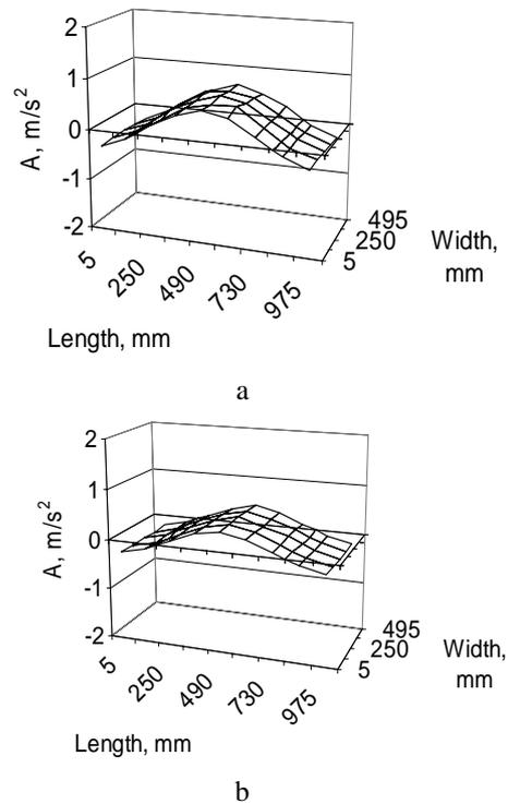
**Fig. 6.** First vibration modes of glued-up panels along grain: a – panel of 5 scantlings ( $f = 152.2 \text{ Hz}$ ); b – panel of 11 scantlings ( $f = 159.6 \text{ Hz}$ )
