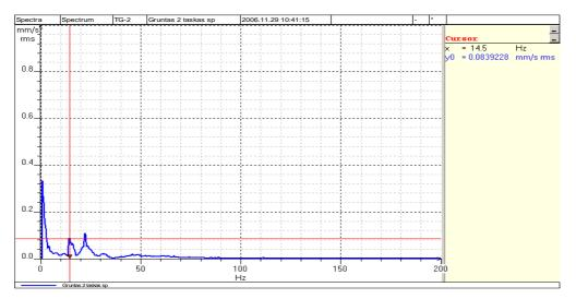
Fig. 3. Vibration spectrum of the ground by the building of the hydroelectric power station
