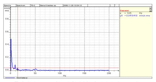
Fig. 4. Vibration spectrum of the wall of the building of the hydroelectric power station
