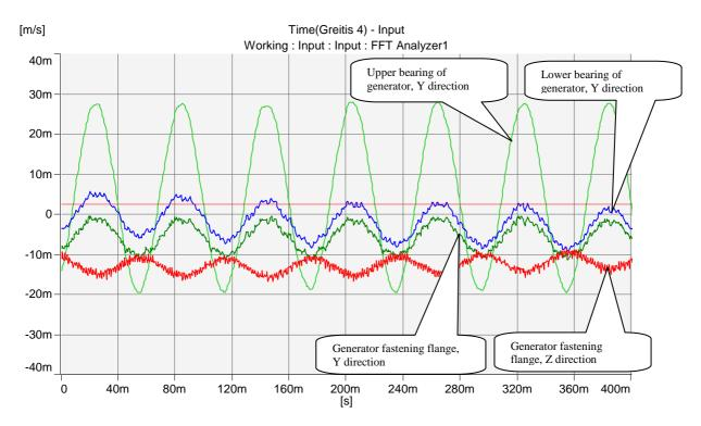
Fig. 5. Oscillograms of the vibrations of generator bearings and fastening flanges of the hydromachinery TG 2
