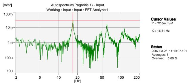
**Fig. 7.** Frequency characteristics of the hydromachinery TG 1. The excitation in the upper point of the generator in the Y direction. The measurement point is the upper bearing of the generator, Y direction.
