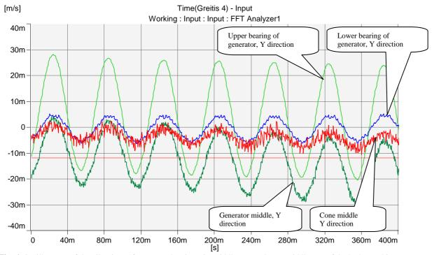
Fig. 6. Oscillograms of the vibrations of generator bearings, its middle part and cone middle part of the hydromachinery TG 2
