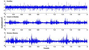
Fig. 2. Vibration signals in different states of compressor
