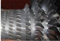
Fig. 2. Broken and worn blades
